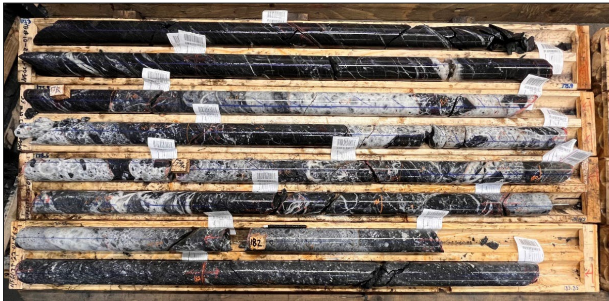
Figure 7-22: Core Photo of Quartz Vein Zone Breccia, Cockade, and Banded Textures within Twin Ponds Drill Hole NFGC-TP-22-01, 173.3 m to 183.85 m
