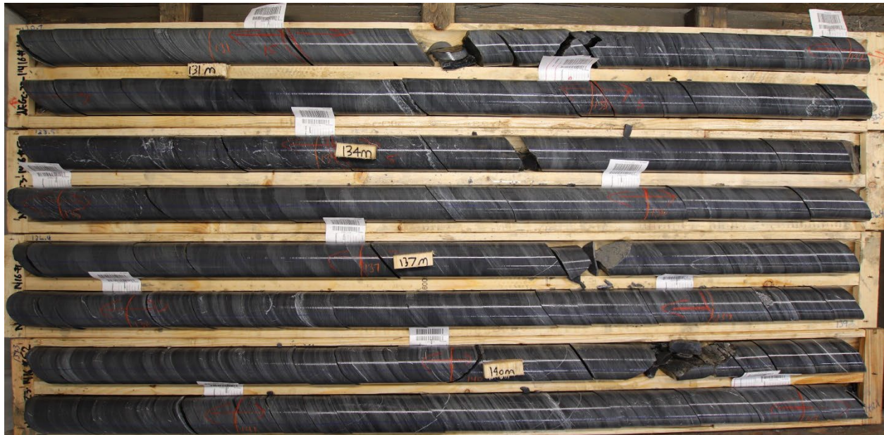
Figure 7-6: Interbedded Siltstone and Greywacke of the AFZ Footwall, Outflow Formation from Drill Hole NFGC-23-1416
