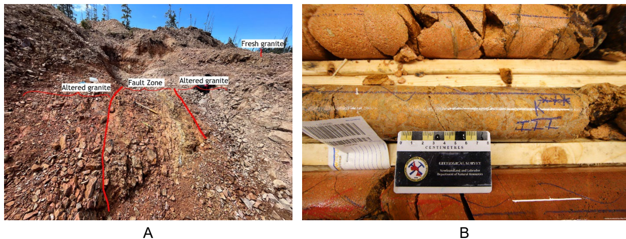
Figure 7-21: Fault Zone in Oxidized Granite (A) and Chalcedonic Quartz Breccia Veins (B) at Mars
