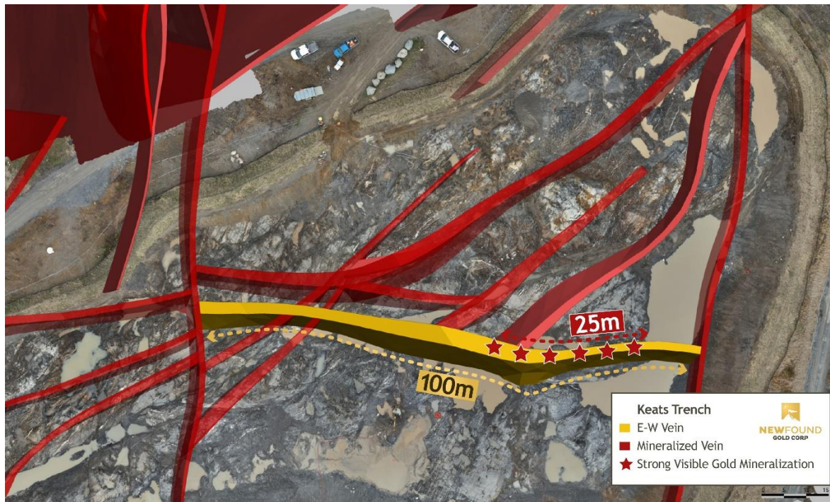
Queensway Project- Keats Trench plan view map with location of strong visible gold mineralization in the E-W Vein (November 17, 2023).
