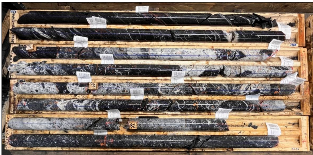
Figure 10.26 Core Photo of Twin Ponds drillhole NFGC-TP-22-01, 173.3m-183.85 m. Quartz vein zone-breccia, cockade, and banded textures.
